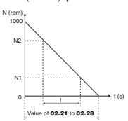
**02.21**: Deceleration rate 1 (main ramp in factory settings) **02.22** to **02.28**: Deceleration rate 2 to Deceleration rate 8
