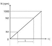
**02.11**: Acceleration rate 1 (main ramp in factory settings) **02.12** to **02.18**: Acceleration rate 2 to Acceleration rate 8
