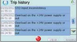
When the drive trips, it is displayed in a red banner, at the top of the interface screen. When the drive trips an alarm, it is displayed in a orange banner.
