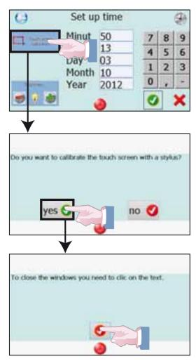
The stylus should then be positioned at several points suggested by crosses positioned on the screen. At the end of calibration, click on the text at the top of the screen to return to the "Date/Time" page.
