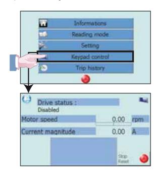
By default, the screen gives Informations about the drive status, the calculated motor speed and the current magnitude. The Stop/Reset command is also active.
