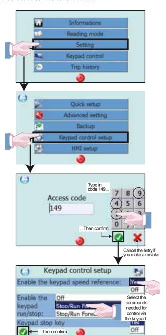
To view the new touch-sensitive buttons that have been enabled, you need to return to the main page, then select "keypad control".
